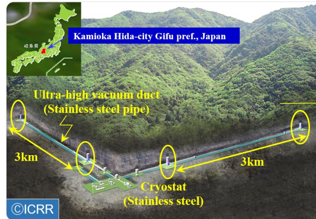
Schematic underground view of the KAGRA facility
