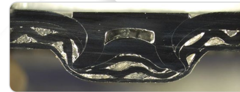
Outokumpu's Stainless Weldable Sandwich offers also a high ability to other joining methods like the mechanical joining process of riveting. Because of the stainless 3D profiled core, the connection results in an outstanding power transmission with an enormous, state of the art not possible compressive rigidity. Background is the possibility to work out an interlocking between the profiled core inside the sandwich and the rivet
