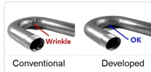
Figure 2: Pipe bending with conventional and developed ferritic stainless steels Picture courtesy of POSCO
