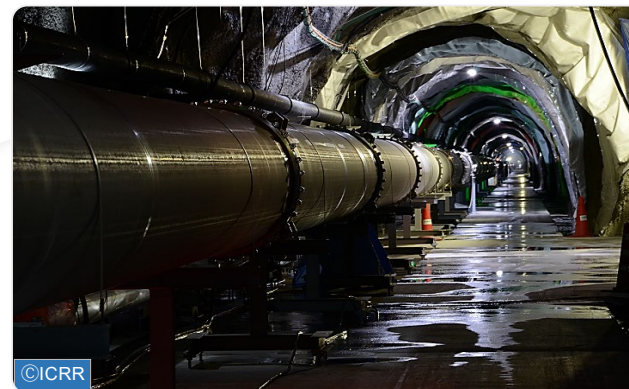
Ultra-high vacuum stainless steel duct of 3,000m in length, as the laser light path in the interferometer
