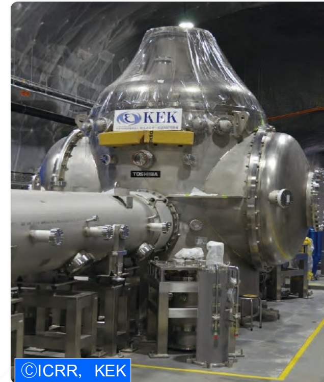
Cryostat (as a container for high purity single crystal sapphire mirror)
